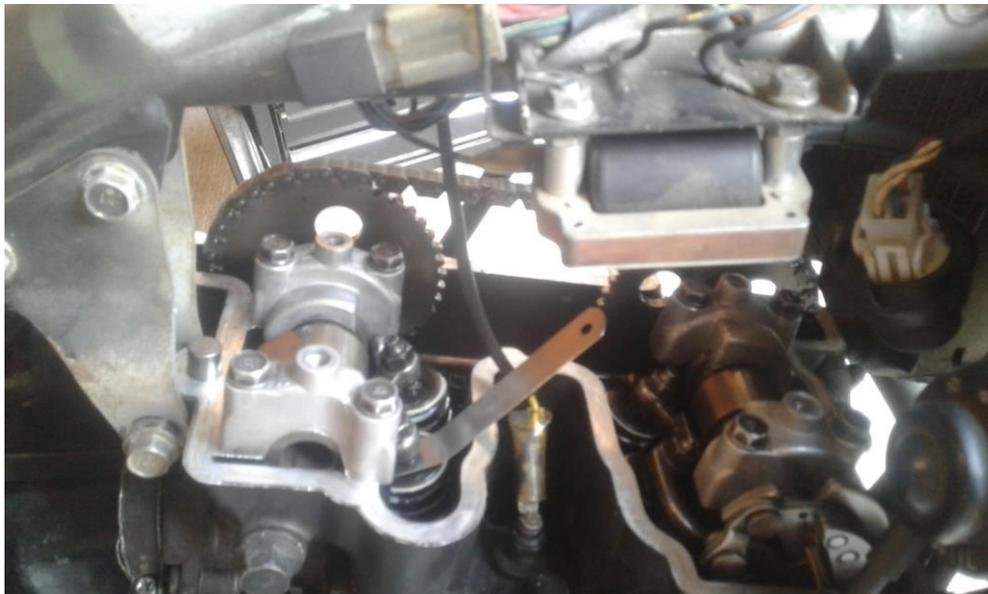
Here is a picture of the four valves with the feeler gauge inserted in one of the intake valves.
