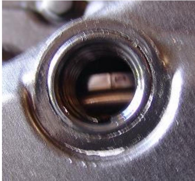
With the engine at TDC the valve clearances were checked with the feeler gauge and all four intake and exhaust valves were still set at 0.009.
