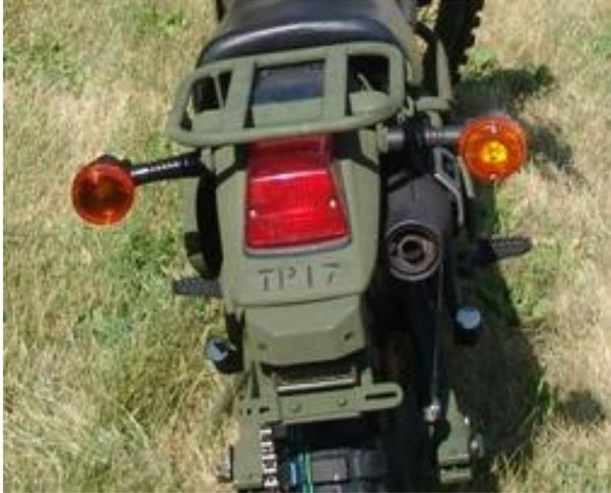
Rear Convoy Rear Light and Brake Light (Above License Plate Mount) and Rear Carrier
