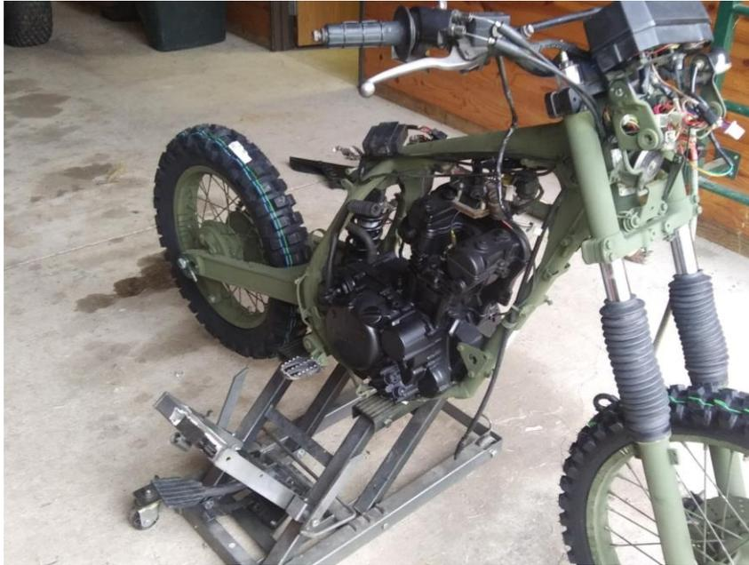
Now the radiators, hoses, carburetor, carburetor cable and choke, air box, clutch cable and engine guards were installed. The front fender, brake caliper and speedometer cable were attached. With that done the front electrical connections were buttoned up, installed front headlight housing, blackout light and front turn signals.
