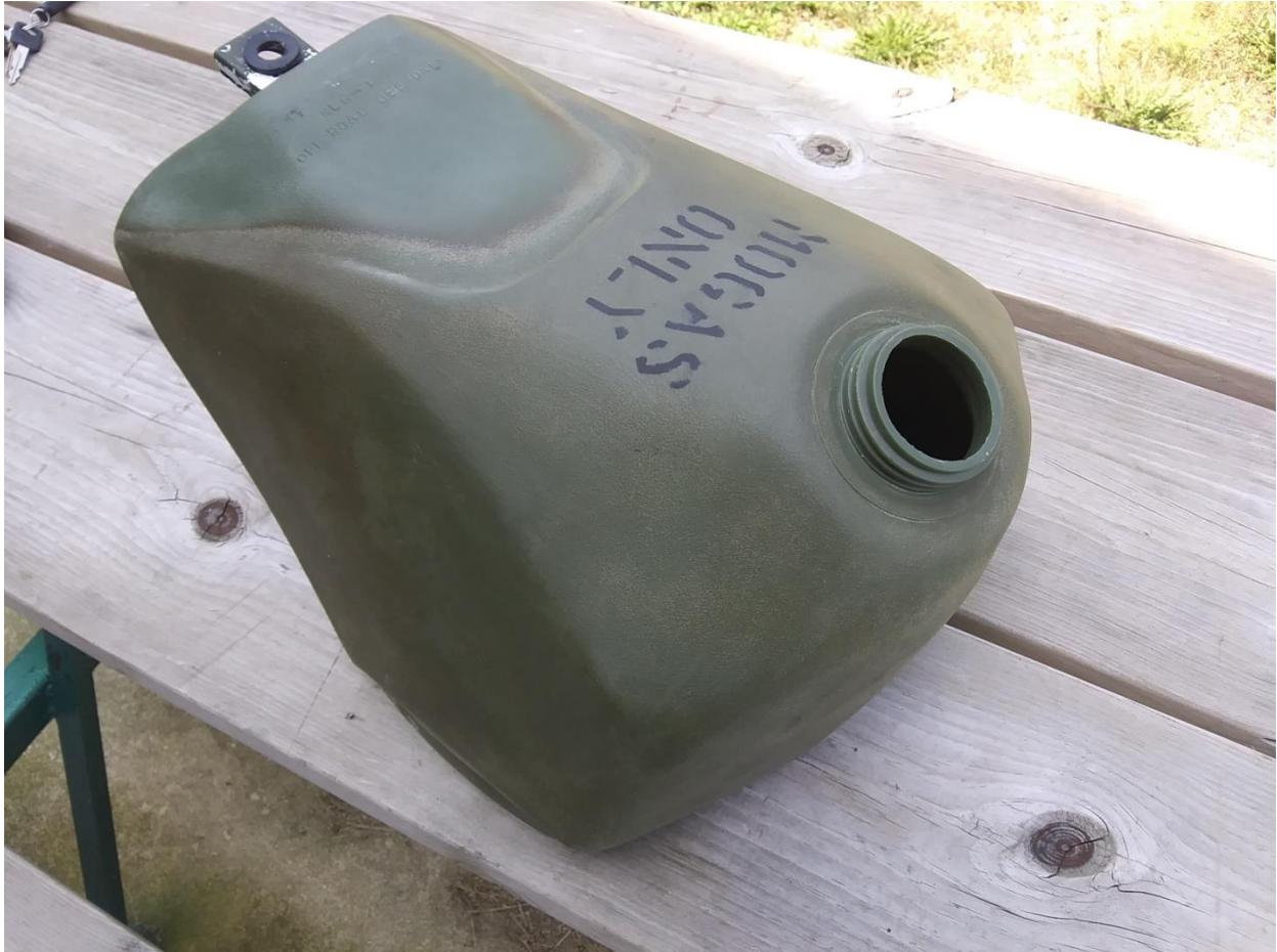
Hayes changed out the fuel tanks on the later M1030's to a larger capacity plastic fuel tank. The Kawasaki stock fuel tank was made of steel and held 2.9 gallons. Hayes purchased their plastic polyethylene fuel tanks from a company who specializes in motorcycle racing plastic fuel tanks. That company is called IMS Products and the replacement fuel tank is rated at 3.2 gallons.
