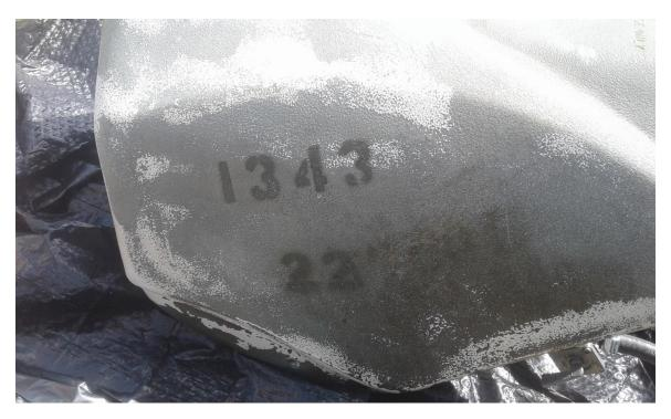
While stripping the white paint off the gas tank the USMC markings were found.
