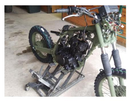
Now the radiators, hoses, carburetor, carburetor cable and choke, air box, clutch cable and engine guards were installed. The front fender, brake caliper and speedometer cable were attached. With that done the front electrical connections were buttoned up, installed front headlight housing, blackout light and front turn signals.
