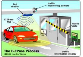
Fig.10: Pervasive Computing Technique in E-Z pass process
