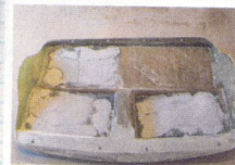
7. The finished structure was cut into a more refined shape. Flat surfaces were created using Evercoat's Tiger Hair fiberglass-reinforced filler.
