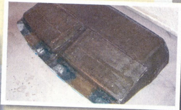
4. The finished structure was "bedded" into the structural ribs in the automobile's roof using Evercoat's Tiger Hair fiberglass-reinforced filler. Eight mounting locations were established, and the structure was held to the roof using eight M8 socket head cap screws (SHCS). Eight rivet nuts, each with pullout strength of 15.7 kN (3,522 pounds), were installed in the roof structure to receive the screws. To prove this console possessed sufficient strength, two adult men, each 778 N (175 pounds), jumped up and down on the structure without any apparent damage.
