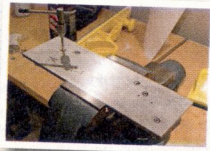
10. Each of the aluminum plates was drilled and tapped with M4 x 0.75 through-holes for mounting audio components and peripherals.
