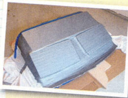
1. The OEM headliner was used as the basis for the mold. High-density fiberboard and duct tape were used to create the basic shape.
