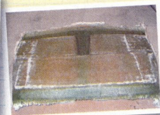
3. To build up the composite structure thickness rapidly, layers of 48-ounce woven roving were used. Layers of Cascade Audio's VB-FD were incorporated into the composite to provide the structure with internal damping.
