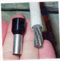
14. Genesis provides these protective ferrules for the power connections. These prevent the setscrew from damaging the fine strands of wire in the cable's conductor.
