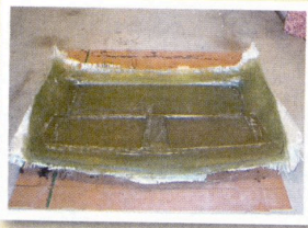
2. The overhead electronics console structure was removed from the mold after about six layers of 6-ounce woven roving were applied using polyester laminating resin.
