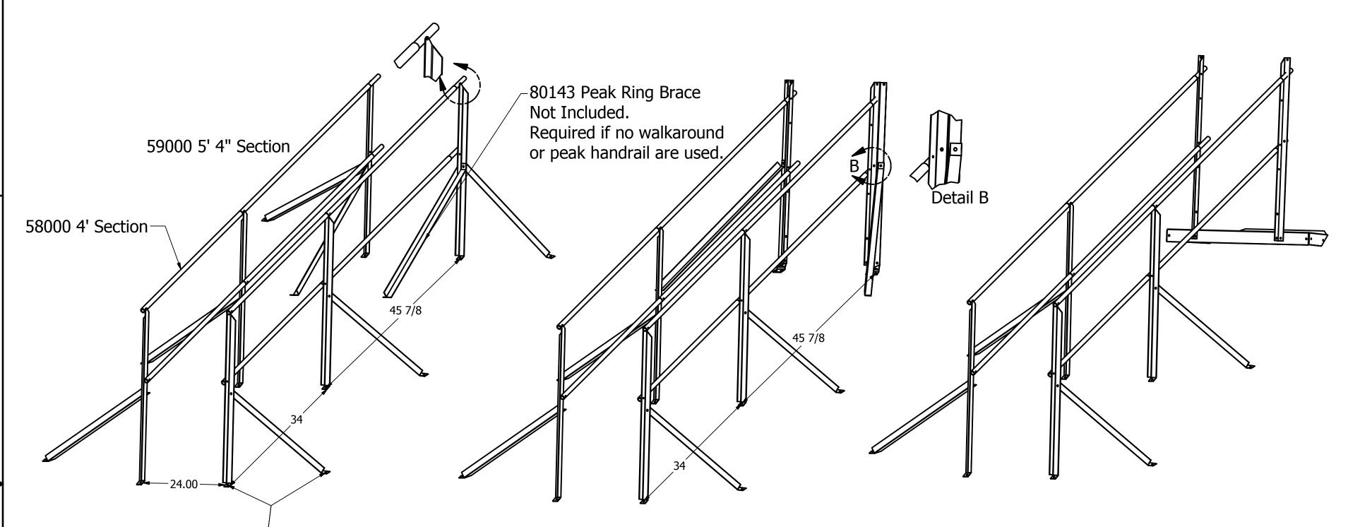
Dimension varies with bin size. – Plumb posts and fasten bracing.
