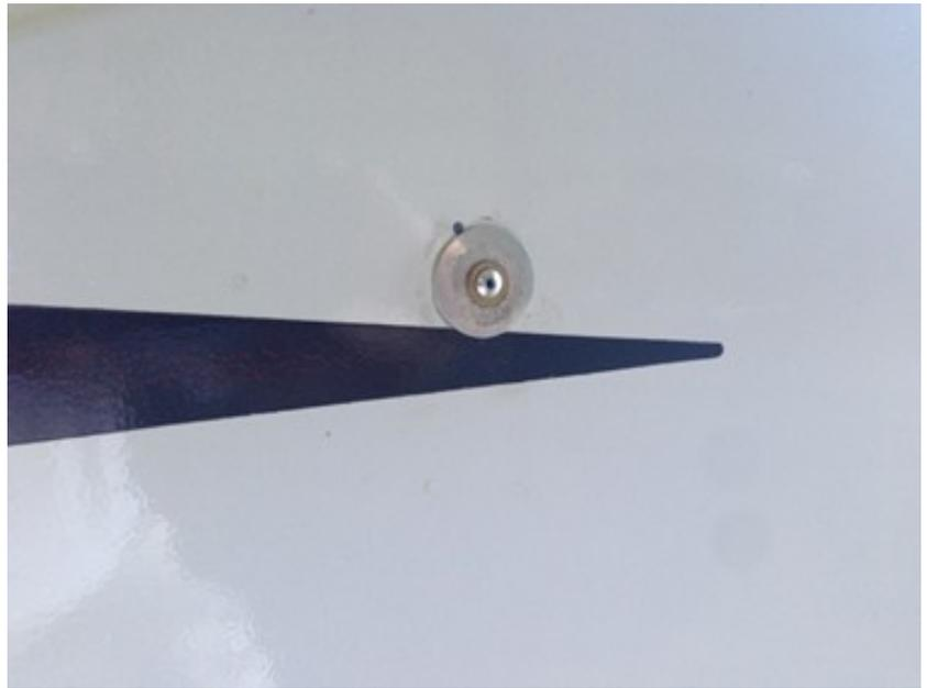
**Static Port Using a Pulled Rivet and Washer**
