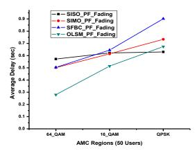
Fig.6d Average Delay for multi-antenna schemes with PF scheduling algorithms for 50 UEs.
