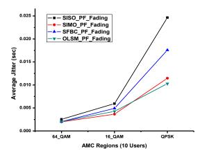
Fig.6c Average Jitter for multi-antenna schemes with PF scheduling algorithms for 10 UEs.
