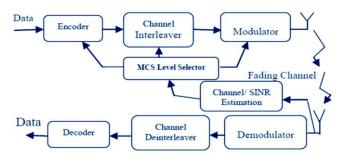
Fig.2: Structure of AMC System [14]
