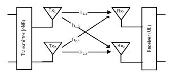
Fig. 4 MIMO with (2x2) Antenna Configuration
