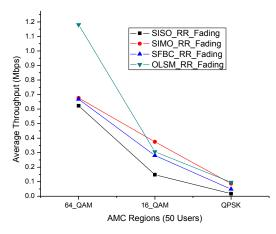
Fig.6e Average Throughput for multi-antenna schemes with PF scheduling algorithm for 50 UEs.
