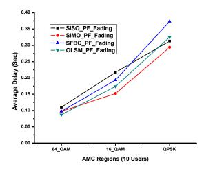
Fig.6a Average Delay put for multi-antenna schemes with PF scheduling algorithms for 10 UEs.
