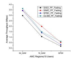
Fig.6b Average Throughput for multi-antenna schemes with PF scheduling algorithms for 10 UEs.
