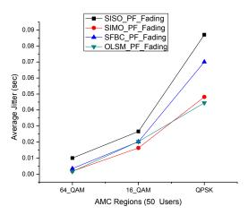
Fig 6f: Average Jitter for multi-antenna schemes with PF scheduling algorithm for 50 UEs
