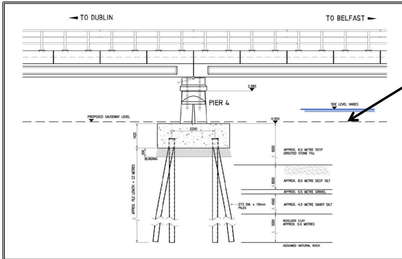
In case scour occurs below this level, the wider seal will create much stronger vortices (U times width) that will scour away rock on sides of seal
