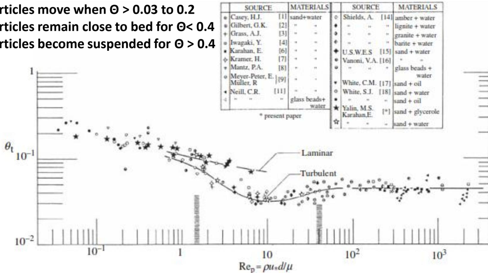
Figure 7.5 Shields diagram for incipient particle motion (Yalin, 1985).
