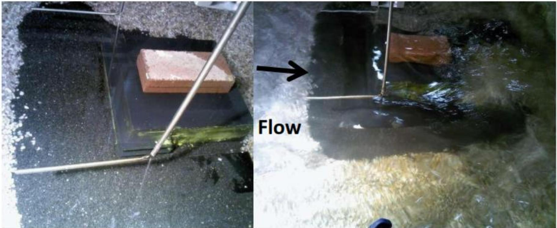
Top view of the scale model of the Bridge Pier Seal with streamlined fairings **BEFORE** test (left) and **DURING** test (right).
