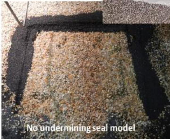
**Note that the streamlined ramps and fairings have prevented scour near and under the seal and downstream.**
