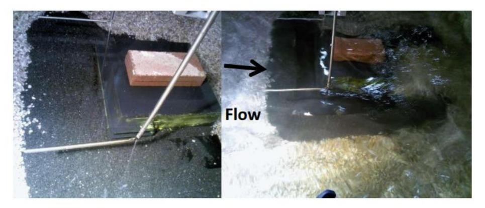
Top view of the scale model of the Bridge Pier Seal with streamlined fairings BEFORE test (left) and DURING test (right).
