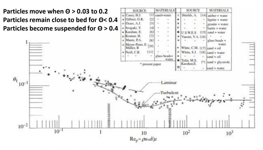
Figure 7.5 Shields diagram for incipient particle motion (Yalin, 1985).
