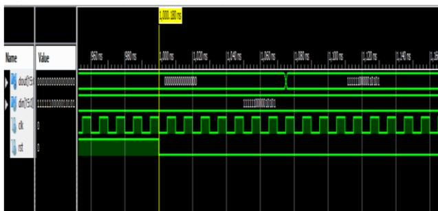
**Fig 7 Simulation Output of Delay8**
