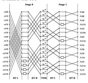
Fig1 Butterfly Structure of 16-point Radix 2<sup>2</sup> FFT
