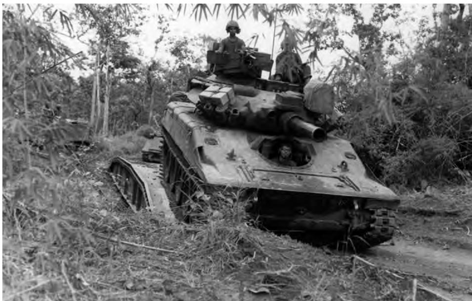
*A Sheridan of the 11th Armored Cavalry crosses an armored vehicle launched bridge.*
