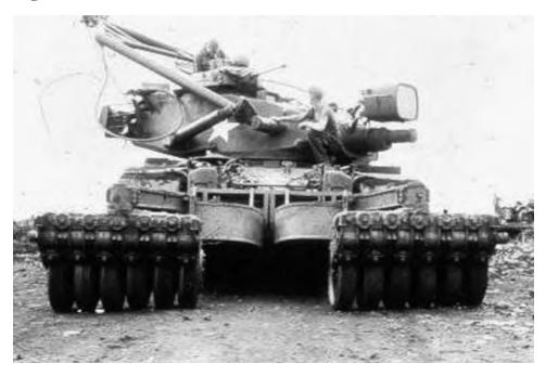
Rollers placed in front of M48 tanks and this combat engineer vehicle expedited clearing roads of mines.
