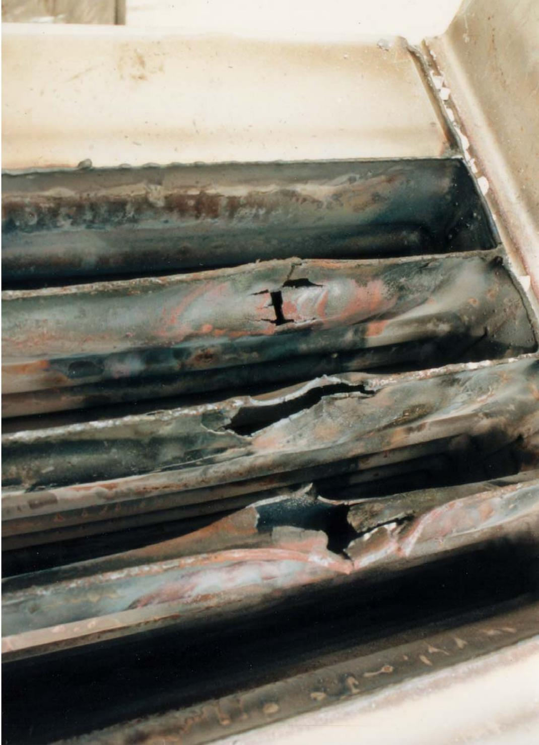
**Photo Seven: Major failure of heat exchanger.**
