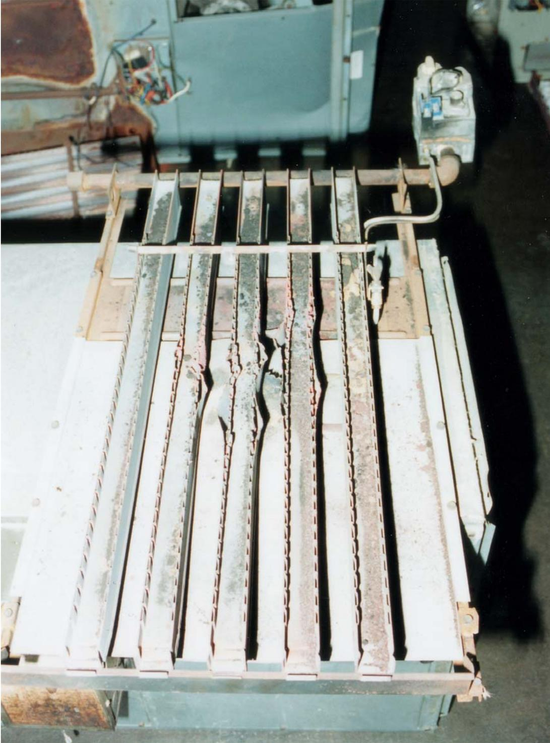
**Photo Six: Failed heat exchanger.**
