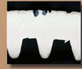
422 Alloy sample 125x magnification. Mounted after 180 days of accelerated formicary corrosion testing, with no through the wall failure.
