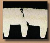
122 Alloy sample 125x magnification. Mounted after 7 days with failure, of accelerated formicary corrosion testing.
