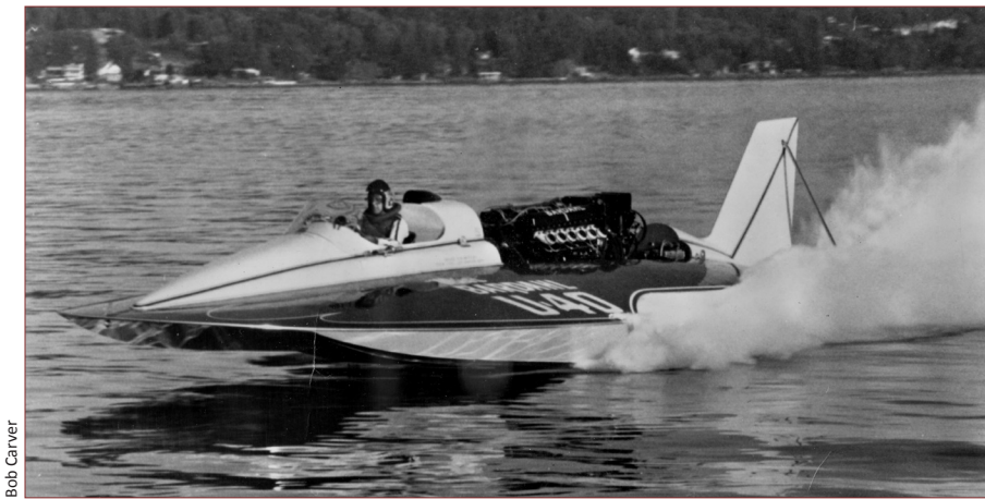
The first unlimited designed by Ron Jones was the ill-fated Miss Bardahl , which featured a cabover design and made its debut in 1966. The boat is shown here during a test run on Lake Washington. When racing in Washington, D.C., early in the 1966 season, the boat suddenly nosed into the water and broke in half, killing driver Ron Musson.
