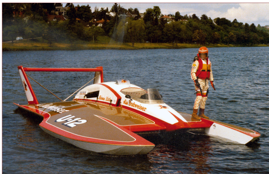
Another innovative boat from the drawing board of Ron Jones was the 1979 Miss Budweiser, shown here after driver Dean Chenoweth completed a test run on Lake Washington. The boat featured a huge Rolls-Royce Griffon engine and a cockpit and engine compartment that was offset to the boat's left side.
