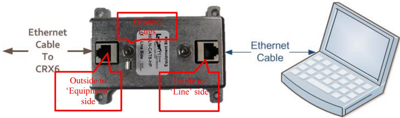
**Figure 4-8: Ethernet Connection for Non-PoE Models**
