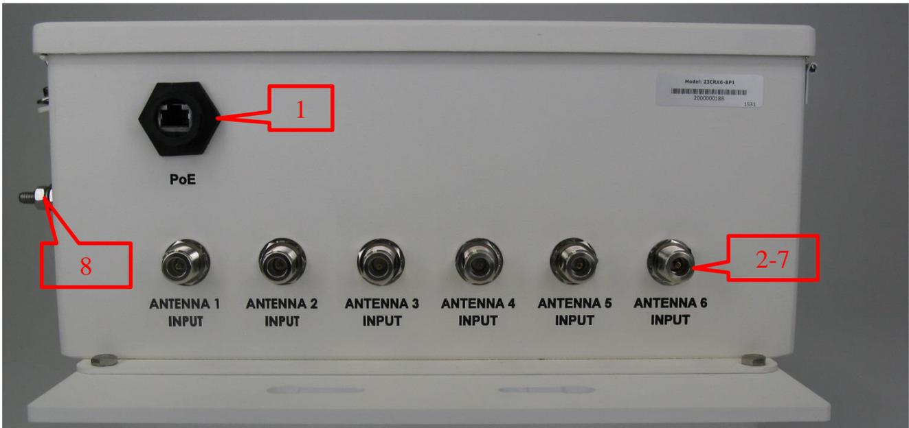
Figure 4-1: Single Channel PoE Connector View
