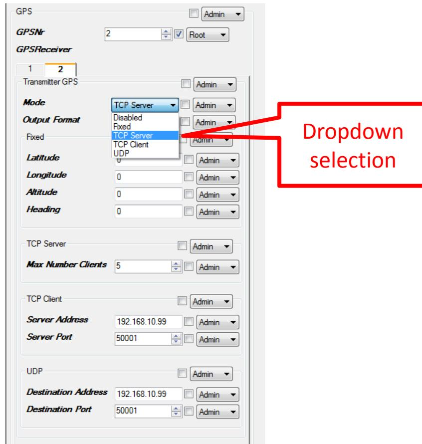
**Figure 5-27: Transmitter GPS Data Output Selection**
