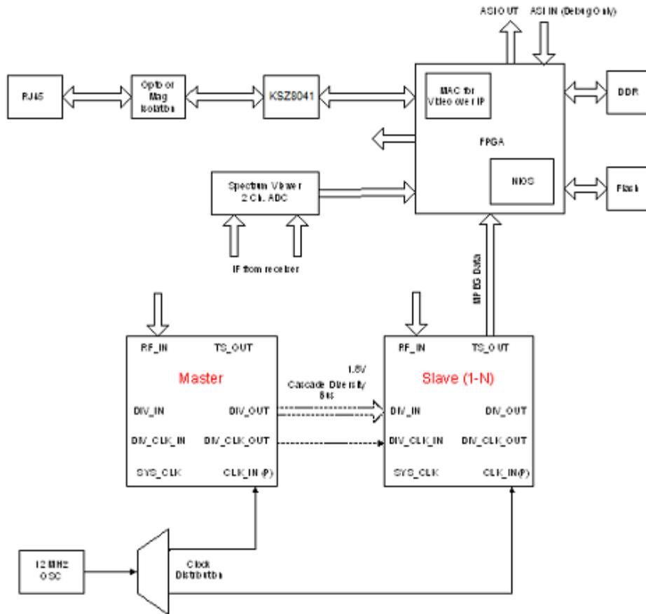
**Figure 2-2: 6 Way Receiver Board Block Diagram**
