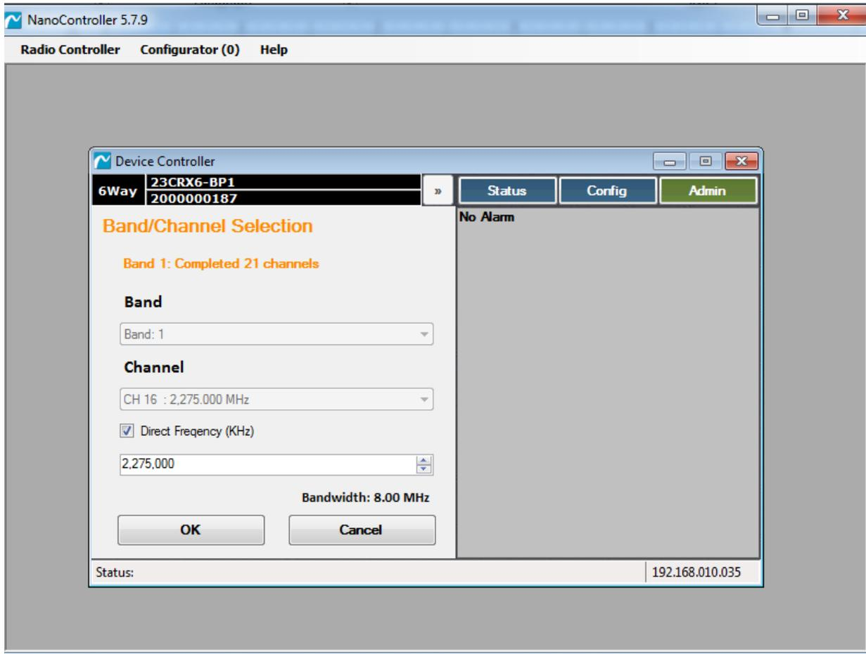
Figure 5-35: NanoController Direct Frequency Entry
