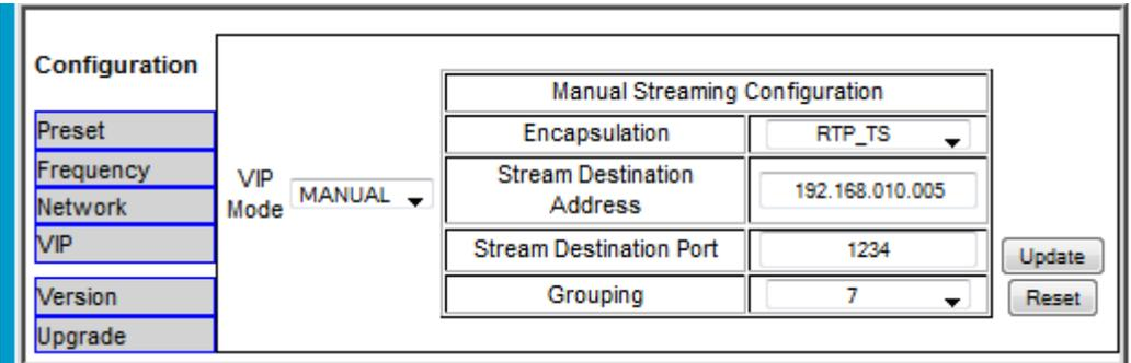
Figure 5-14: Manual Streaming Configuration
