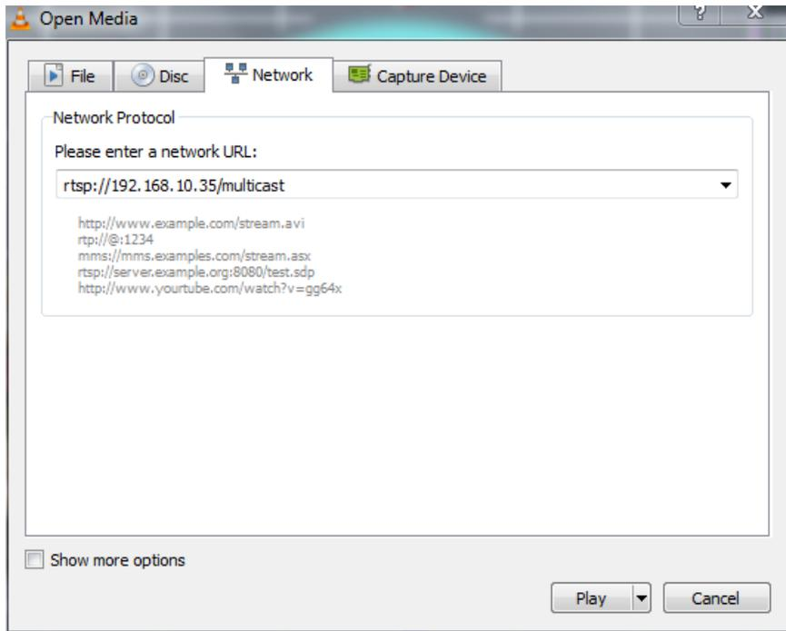
**Figure 5-23: VLC configuration RTSP Multicast, RTP**
