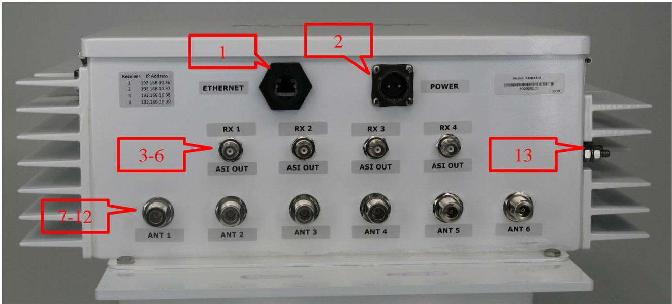
**Figure 4-2: Multi-Channel, Ethernet, Power and ASI Option**
