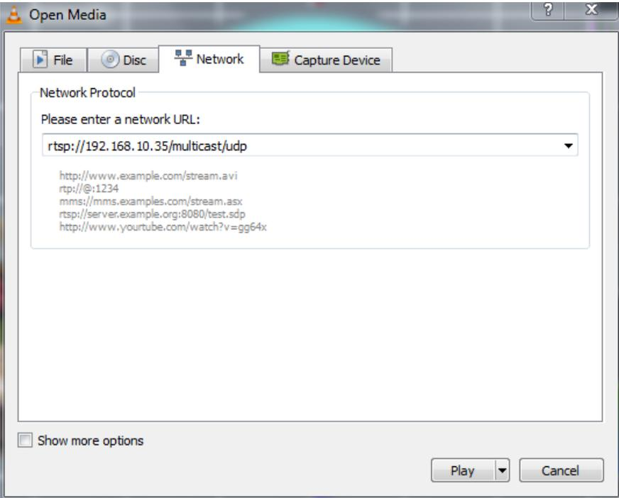
Figure 5-24: VLC configuration RTSP Multicast, UDP
