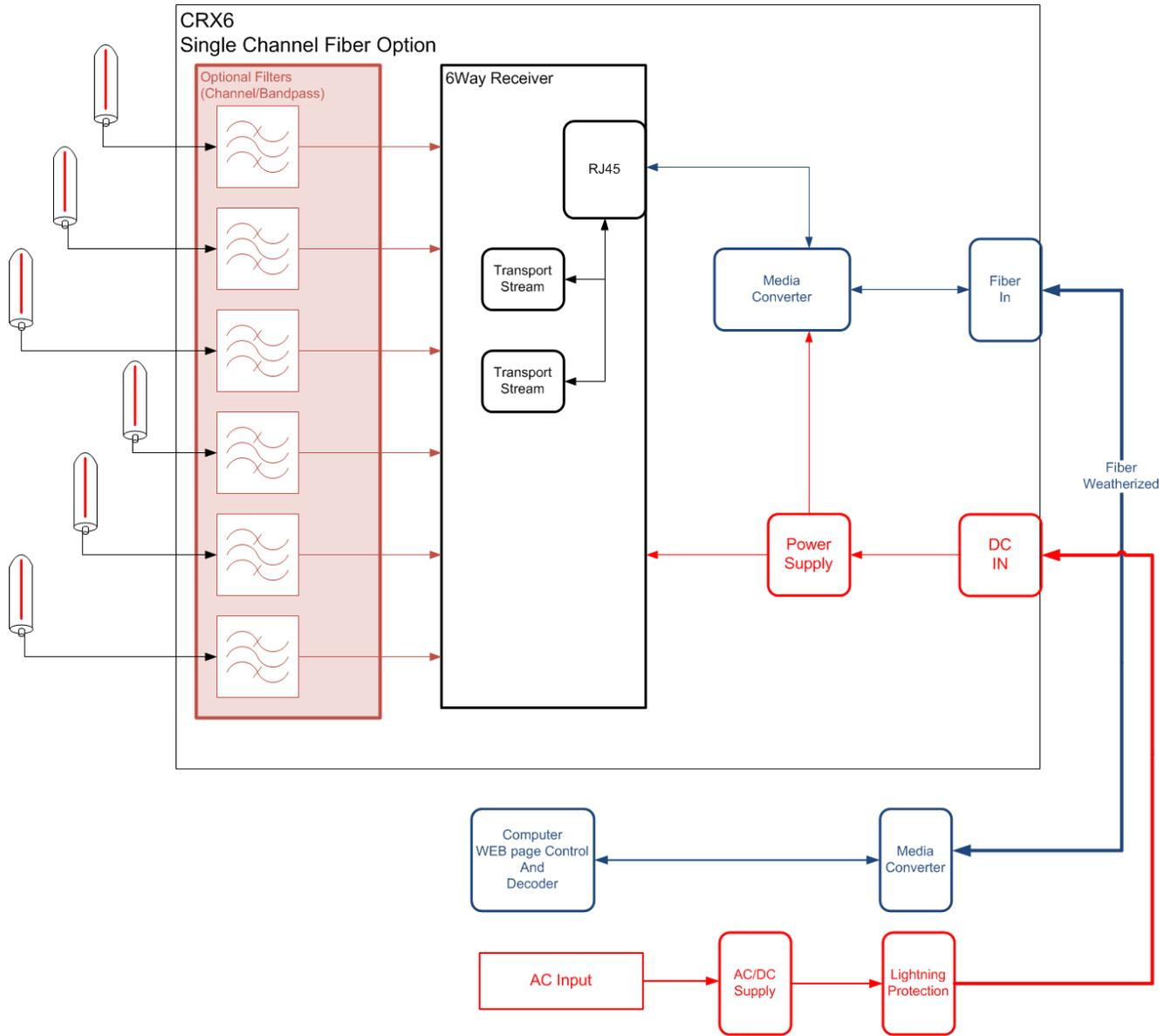
**Block Diagram 2-2: Single Channel with Fiber**
