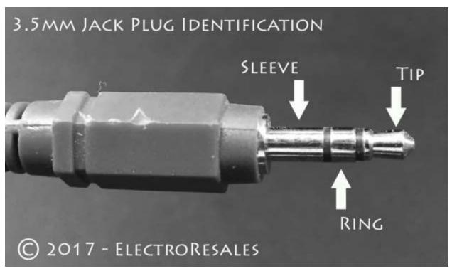
The Dit & Dah contacts are connected to the Tip and Ring, while the common is attached to the sleeve. A stereo audio jack cable should work well, you may need to use an adapter plug on one end depending on your key unit, consult the keys user manual. Most keying units allow the paddles to be swapped either in software or by physically moving a header or switch. Again consult your keying unit manual for help on this.
