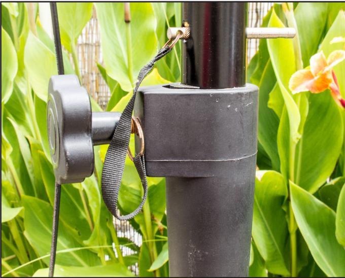
Figure 21. The securing knob on the tripod showing the pin inserted to extend the mast height.
