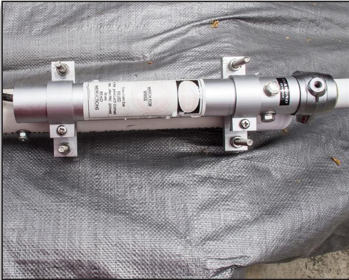
Figure 16. Antenna base inserted into mounting brackets.
