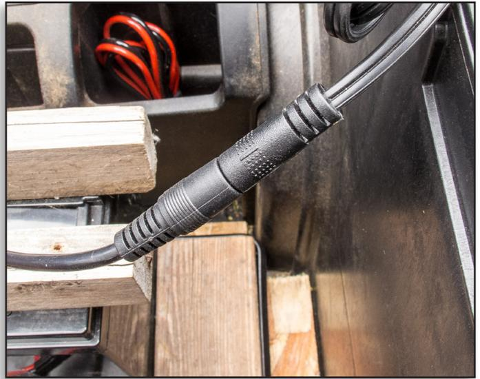
Figure 26. Close up of the Bioenno charger connected to the battery.
