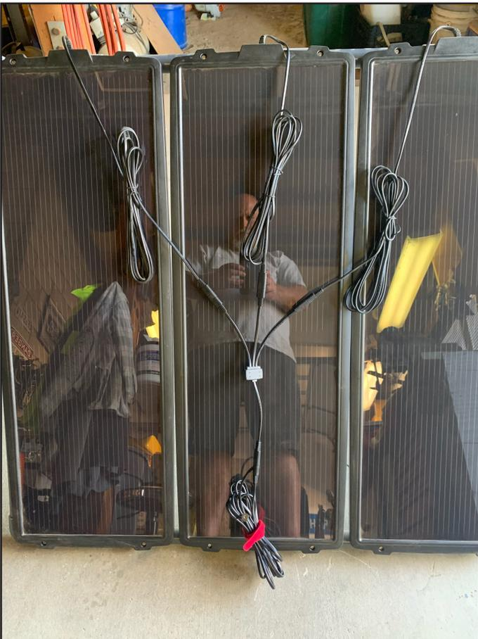
Figure 27. Harbor Freight three-panel solar charging system.
