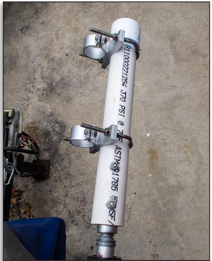
Figure 14. PVC painter's pole extension and antenna mounting bracket.
