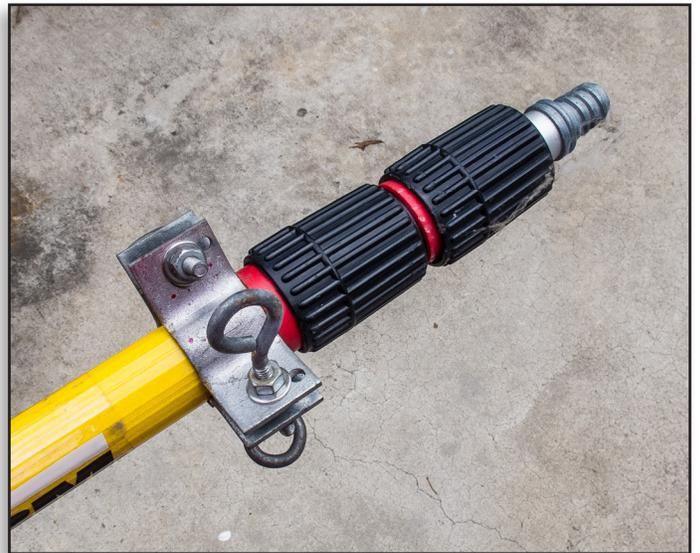
Figure 12. Top of painter's pole mast with guying ring.
