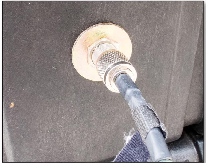
Figure 10. Coaxial cable connector on the rear of the radio box.
