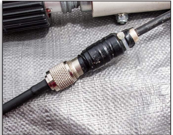
Figure 18. Coaxial cable connected to antenna pigtail.
