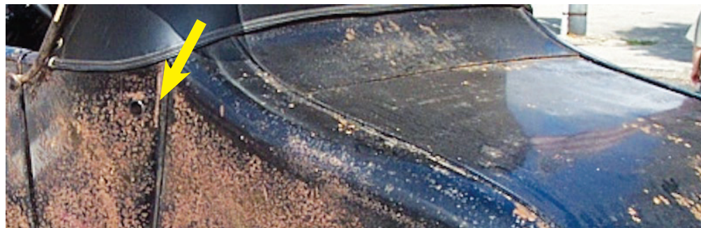
Original runabout with remains of welting between body and deck
