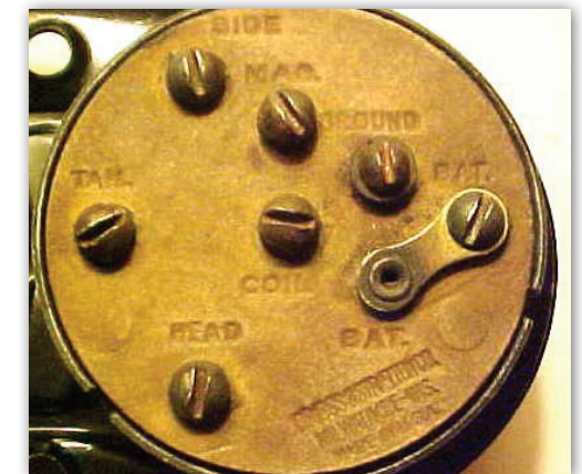
Terminals on switch plate. Note the "Ground" terminal does not have a purpose other than in testing, as noted in the Ford Service Bulletin instructions above.
