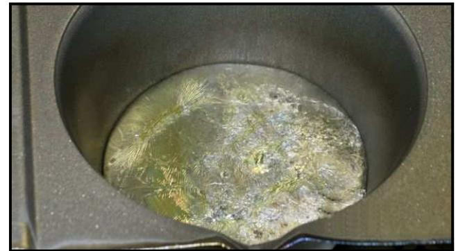
Melted bismuth showing the yellowish slag floating in the top of the liquid. The slag can be removed with a stainless steel kitchen fork.
