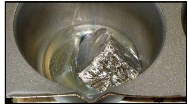
Melting bismuth in a cupcake pan. The pan has been cut apart and a pour spout has been bent into one side.
