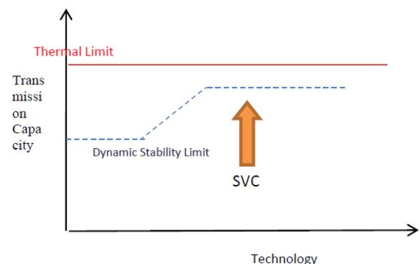
Basic SVC control strategies are examined in terms of enhancing the dynamic and transient stabilities, improving transmission capacity and damping power oscillations.
