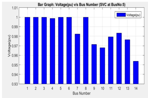
Fig.8. Voltage profile of IEEE 14-bus test system with and without SVC
