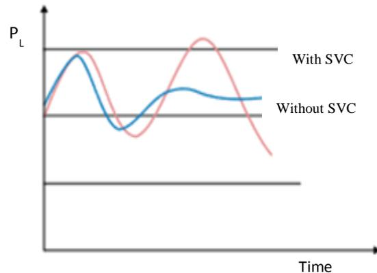
SVC is connected in shunt and its output can be capacitive or inductive current to the system that it is connected. It is used for controlling reactive power and it can be used as a switch or as a continuously controlled valve by controlling the firing angle. With static VAR compensator, we find stability, security, controllability and high-quality electric power. [5]
