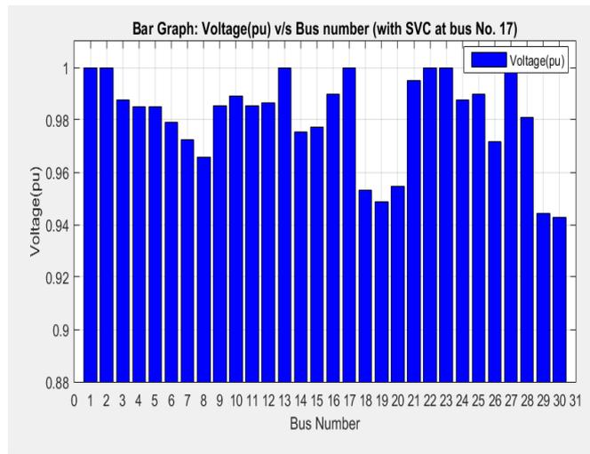
Fig.13. Voltage profile of IEEE 30-bus test system with and without SVC
