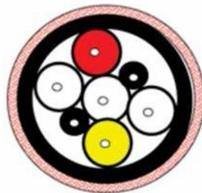
Figure 2: TT5000 sensor cable cross section
