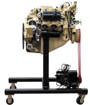
H-HMMWV-6.2-CA Engine Cutaway on Mobile Stand
