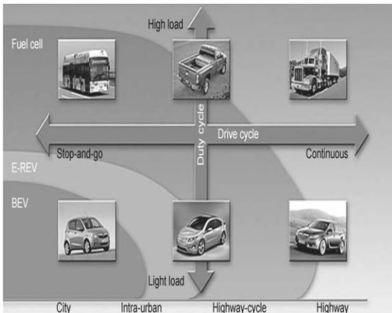
Figure 2. Application map for various EV technologies.
