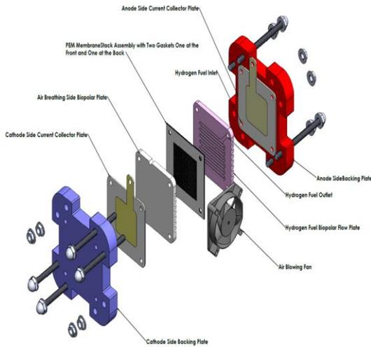
**Figure 1. The polymer electrolyte membrane fuel cell (PEMFC).**
