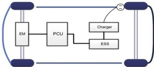
Figure 3. Drive train schematic diagram of BEV's.
