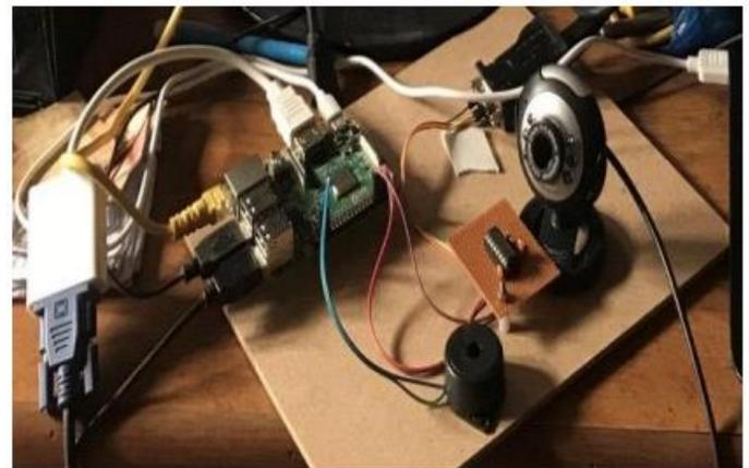
Figure 2: Raspberry Pi with a buzzer
