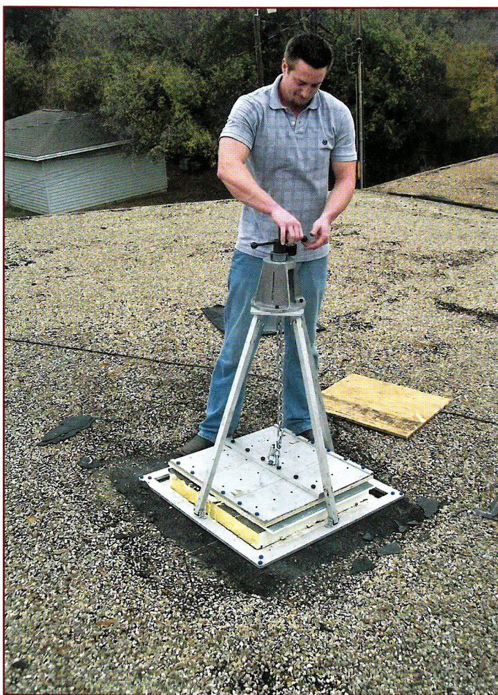
Figure 2. A worker performs a bonded test of rigid board insulation adhered to the substrate in accordance with ANSI/SPRI IA-1 2021 version. 10
