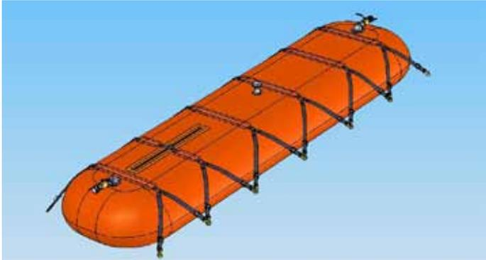
The BATT's complex buffering system is designed specifically for fluid travelling inside an aircraft.
