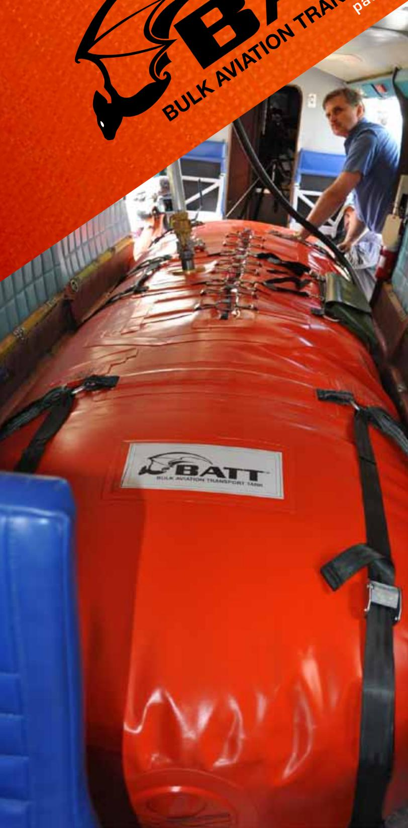
SEI's award-winning bulk aviation transport tank is the world's first double-walled, baffled fuel transportation tank. Each tank is designed specifically for the aircraft using it to ensure a precise fit and to maximize the load-carrying capacity of the aircraft. Bulk fuel aviation transport tanks are made from two main components: a heavy duty, abrasion-resistant outer tank (with a built-in strapping system that also serves as secondary containment) and a fuel-specific, baffled inner tank.
