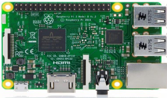
Fig.3: Raspberry pi Board
