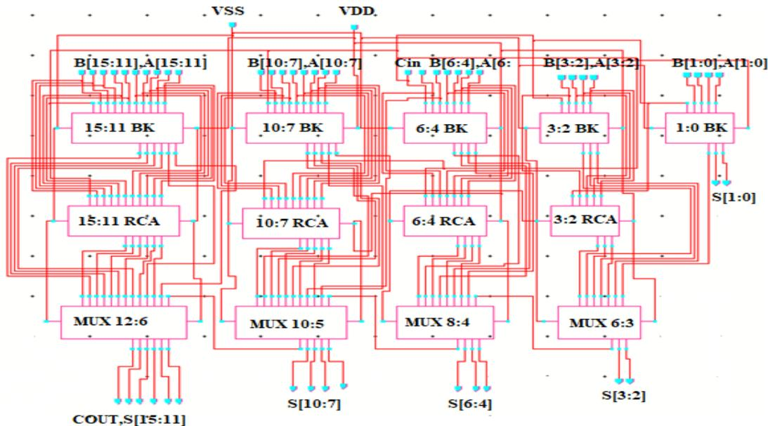
Fig.4: The schematic diagram of 16-bit Regular SRBK CSA
