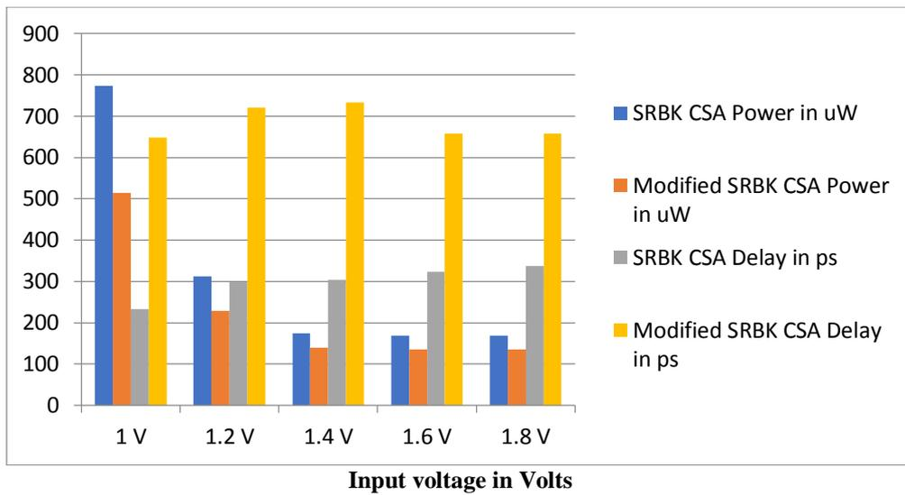
Fig.8: Comparison of Regular SQRT BK CSA and Modified SQRT BK CSA of 8-Bit for power and delay comparison at different input voltages
