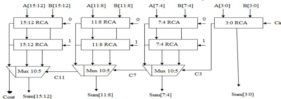
Fig.2: 16-bit conventional carry select adder
