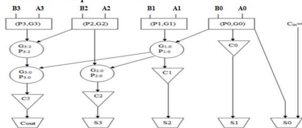
Fig.3: Block Diagram of 4-Bit Brent Kung Adder
