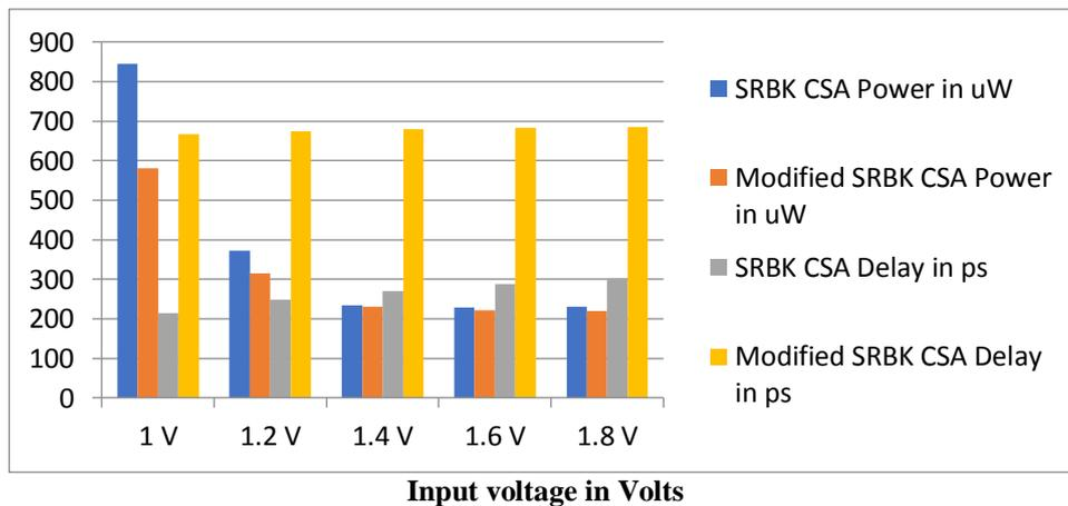
Fig.9: Comparison of Regular SQRT BK CSA and Modified SQRT BK CSA of 16-Bit for power and delay comparison at different input voltages
