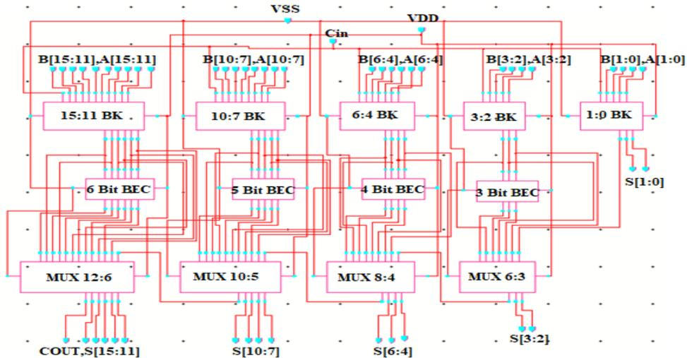
Fig.6: Schematic of 16-Bit Modified SQRT BK CSA
