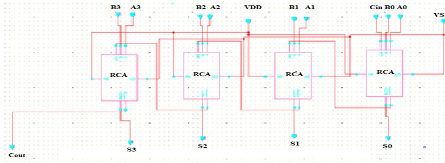
Fig.1: 4-bit Ripple Carry Adder
