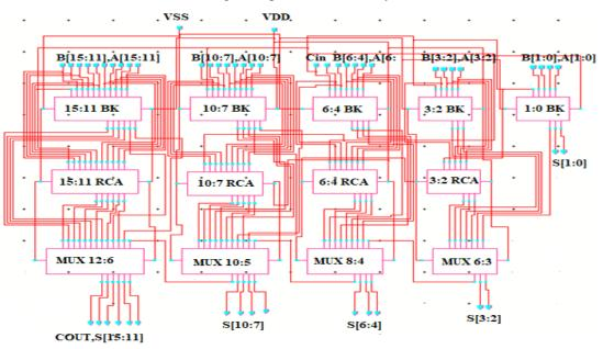
Fig.4: The schematic diagram of 16-bit Regular SRBK CSA
