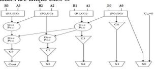
Fig.3: Block Diagram of 4-Bit Brent Kung Adder
