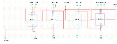
Fig.1: 4-bit Ripple Carry Adder
