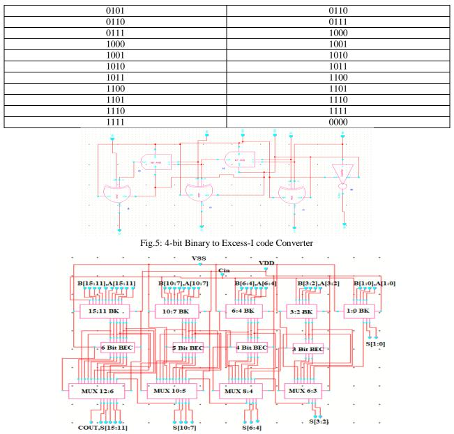
Fig.6: Schematic of 16-Bit Modified SQRT BK CSA
