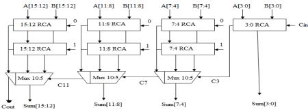
Fig.2: 16-bit conventional carry select adder
