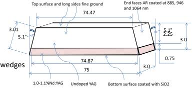
COATING Both wedged end faces AR coated at 885 nm, 946 and 1064 nm, 5.1° AOI Bottom surface coated with 1-3 µm layer of SiO2.
