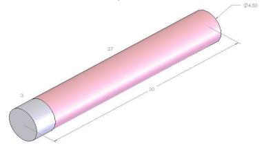
COATING Both 4.5 mm dia. ends R</= 0.5% @ 808nm, R</= 0.1% @ 1064nm
