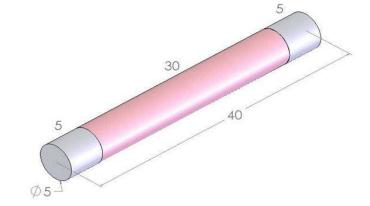
**COATING** Undoped YAG: R>99.9% @ 1064nm, Tav>97% @ 790-820nm, AOI = 0-50º Nd:YAG: R<0.15% @ 1064nm, Tav<3.0% @ 790-820nm, AOI = 0-15º
