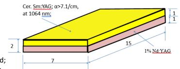
COATING Both 2mm x 15mm surfaces AR/AR R<0.2% at both 1064 and 1340 nm; AR/AR 808 R<1%; LIDT >10 J/cm2 at 1064nm; 10 ns, 10Hz
