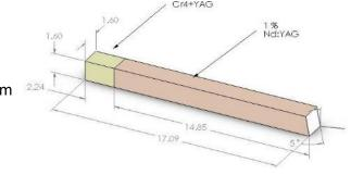
**COATING** Cr4+:YAG end (1.6 mm x 1.6 mm): R = 60% +/-3% @ 1064nm
