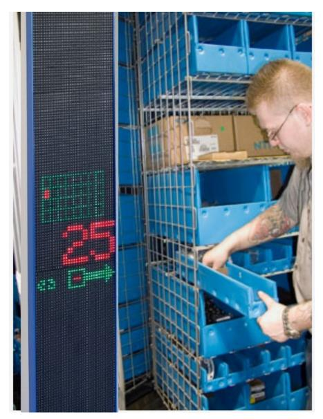
PLT is a modern Pick Light Tower for Horizontal Carousel Applications. The PLT displays information including carousel status, carousel carrier number, transaction quantity and also shows the transaction location on a flexible grid display that matches the actual picking containers. The Tower is available in various heights from 8..12ft and is filled with full color LEDs from top to bottom for complete flexibility to match your shelving on the carousels.
