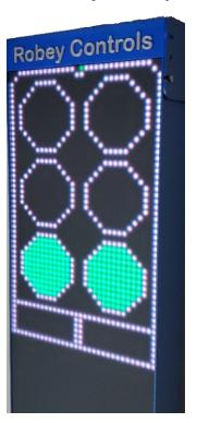
The Black Acrylic LED cover gives a beautiful contrast to the face of the PLT and makes it easier for cleaning but does dim the LED brightness a bit.
