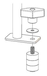
The threads of the Anchor Assembly will fit up into the holes. Replace the Washer and T-Knob. Screw the T-Knob and Washer down until it is finger tight but can still spin freely in the hole.
