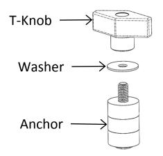
Remove the T-Knob and Washer from each of the Twist Lock Anchor Assemblies.
