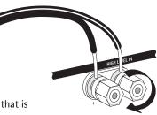
**NOTE:** When making high level connections be sure to maintain proper polarity - that is connect + to + (positive) to (positive) and - to - (negative) to (negative). All wire has one of its conductors marked in some way to make it easy to trace the connections. Typically there is a stripe on the insulation or a rib molded into it. Or the insulation will be transparent and the wire strands of one conductor will be copper colored and the other will be silver colored.
