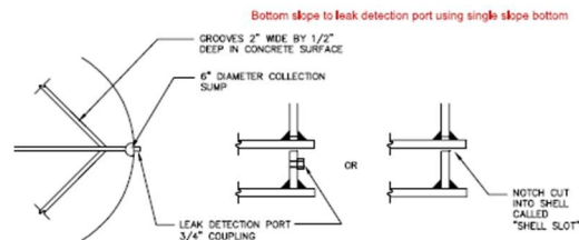
Figure 3 Double Bottom Design Details
