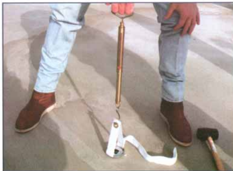
Photos 3 and 4: A spring-type (fish) scale (left) and a custom-fabricated sheet metal holding clamp (right) may be used for pull-out resistance tests on base sheet fasteners.
