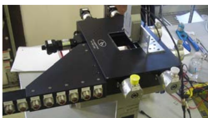
Figure 4: Slit system linear positioning testing.
