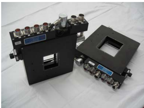
Figure 5: Custom High Precision Slit system delivered to ANSTO.
