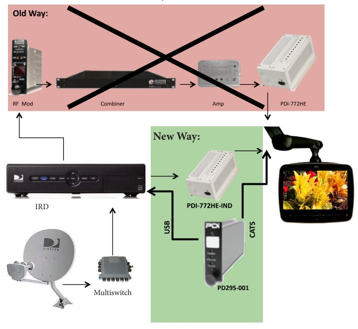
The PD295-001 DIRECTV® satellite interface mini-mod by PDi or the universal infrared version PD295-002 each:
