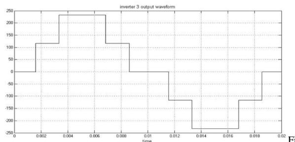
Fig. 13 Inverter 3 resultant output voltage waveform
