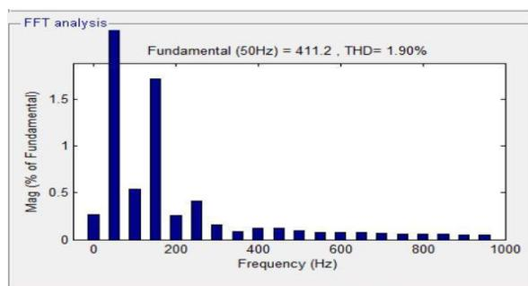
Fig. 20 THD of newly proposed system with LC filter
