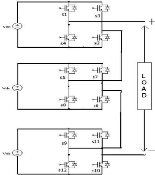
Fig. 1 Seven level inverter block diagram
