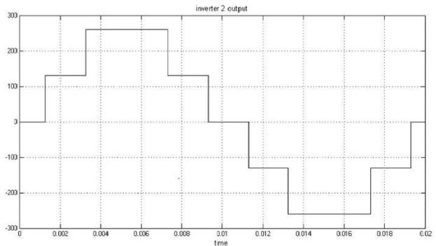
Fig. 8 Inverter 2 resultant output voltage waveform
