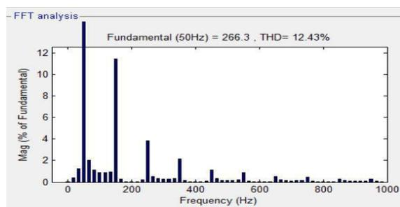
Fig. 19 THD of newly proposed system without LC filter
