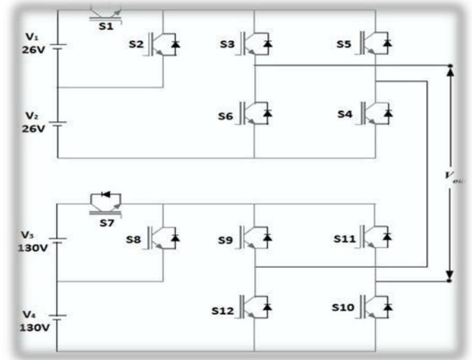
Fig. 2 Proposed 25 level asymmetric multi-cell CMLI
