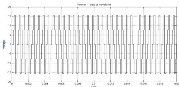
Fig. 11 Inverter 1 resultant output voltage waveform
