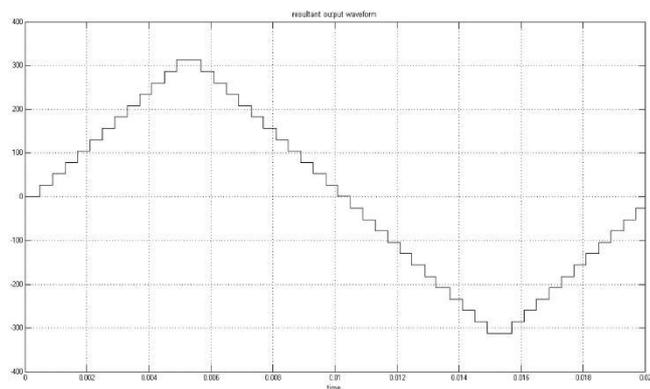
Fig.9 25 Level Resultant output voltage waveform
