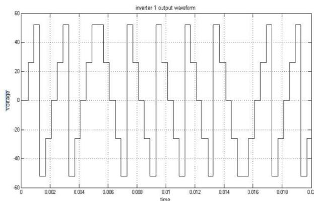
Fig. 7 Inverter 1 resultant output voltage waveform
