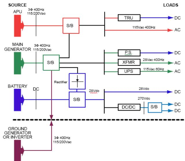
Fig.1 Structure of Aircraft Power System
