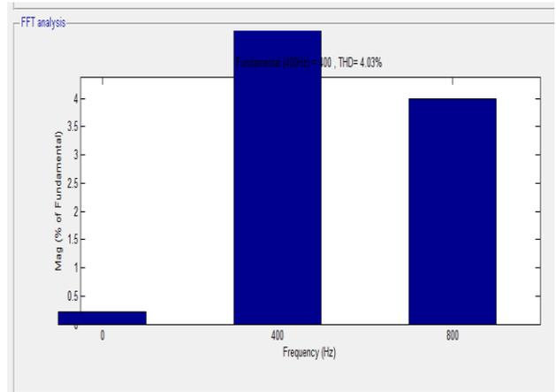
Fig.11 Harmonic Spectrum Of Source Current Without APF
