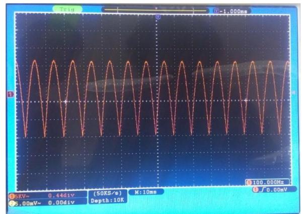
Fig.18 Digital CRO waveform of Sag voltage.
