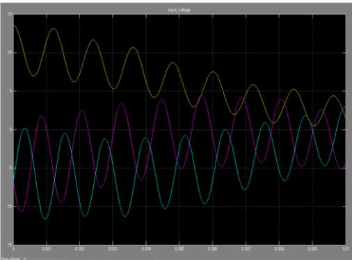
Fig.9 Source Current Without Active Power Filter
