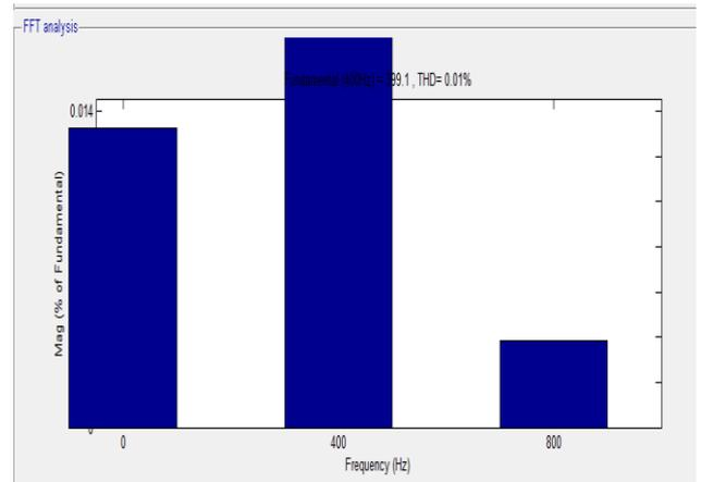
Fig.12 Harmonic Spectrum Of Source Current With fuzzy based APF
