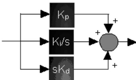
Fig.4 Representation of PID
