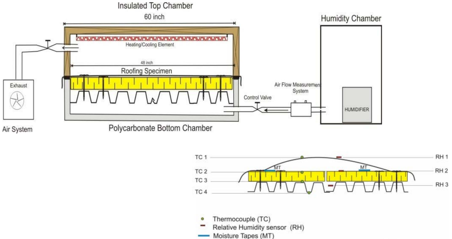
FIGURE 22: INSTRUMENTATION FOR TEMPEARTURE AND RH MONITORING
