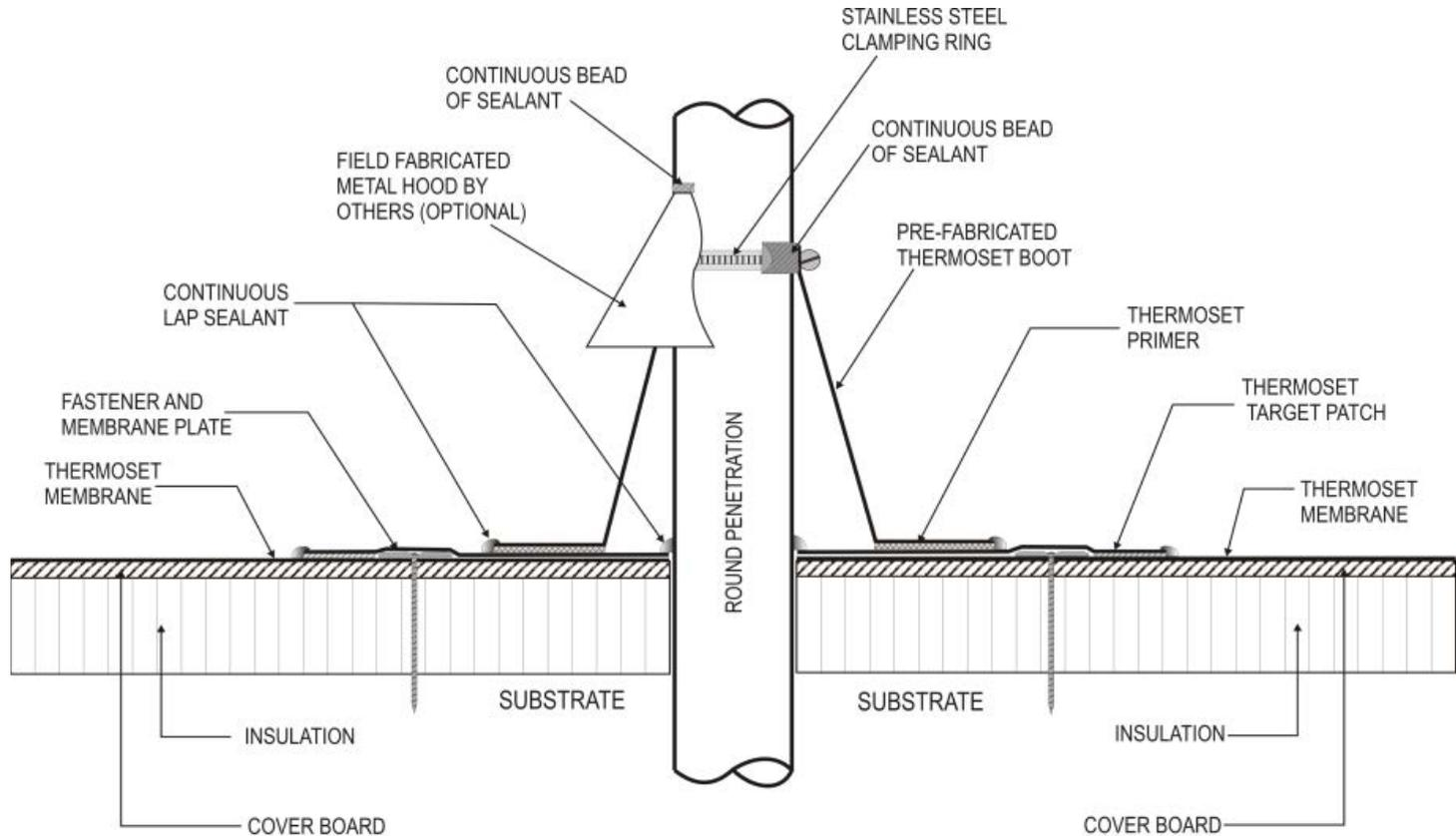
TYPICAL PRE-FABRICATED PIPE BOOT FOR THERMOSET MEMBRANES
