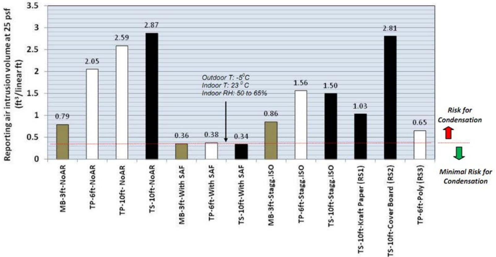
FIGURE 29: AIR INTRUSION LIMIT FOR POTENTIAL CONDENSATION IN THE ROOFING SYSTEM
