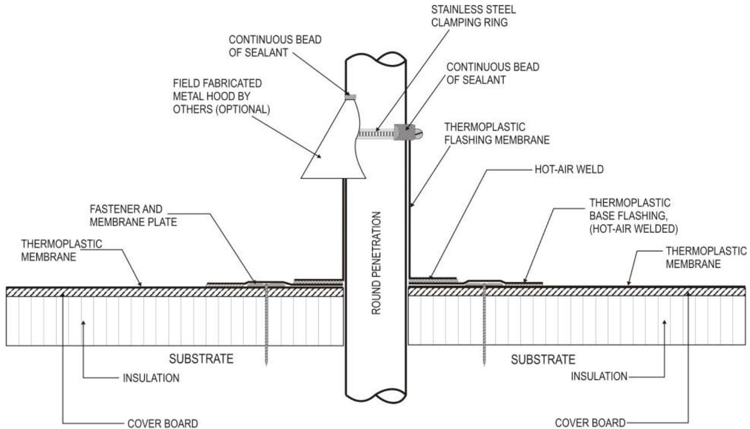
TYPICAL FIELD FABRICATED PIPE FLASHING FOR THERMOPLASTIC MEMBRANES
