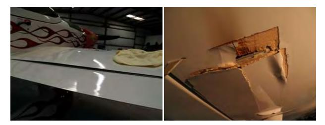
These photos show the wing trailing edge and the bottom area under the fuel tank.
