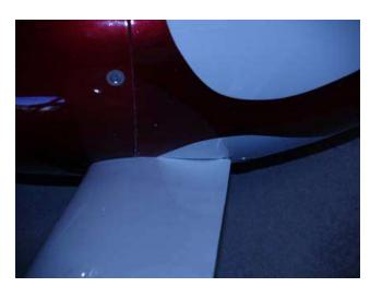
I like the fit and the fairing is very secure. Originally I had made the fit very tight causing the wheel pants to slightly bend with pressure against the fairing. Rubbing is not good as it turns into holes so I took off the pressure and gave some clearance for movement. Let you know if it works.
