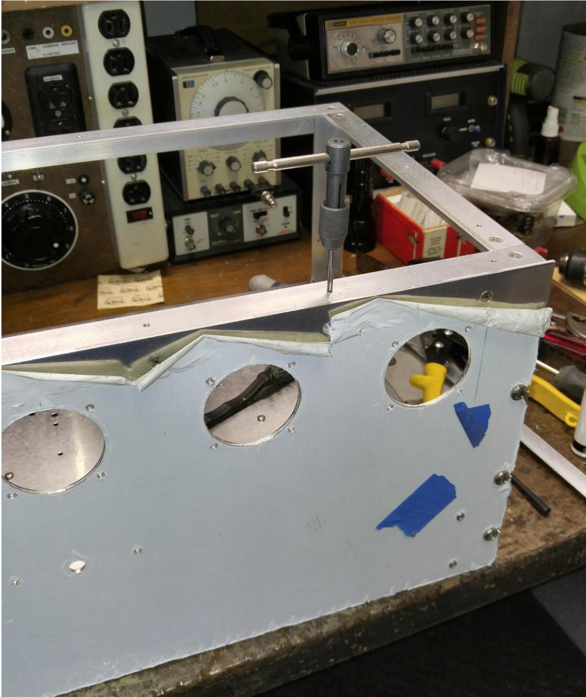
**Figure 4: Tapping Holes in Cabinet Frame**
