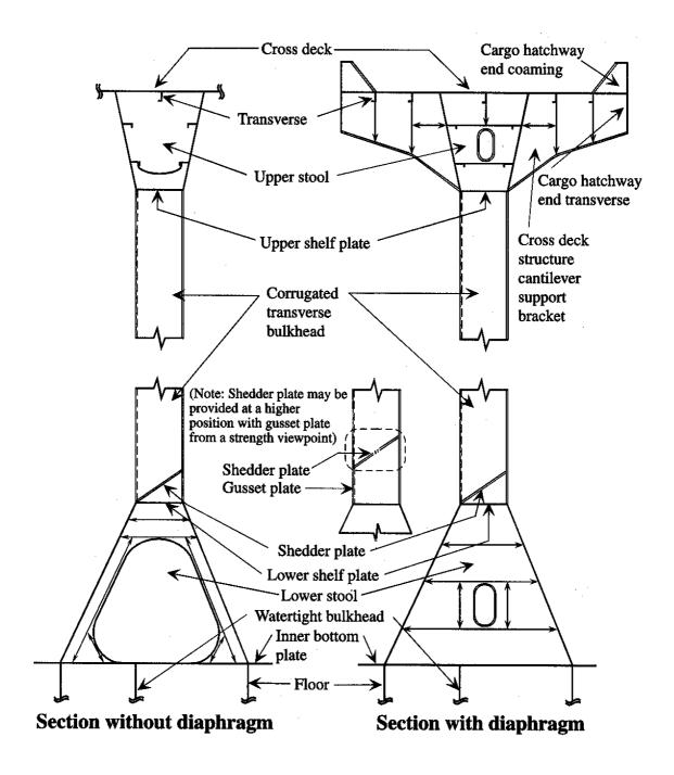
Figure 7: Bulk Carrier — Typical Transverse Watertight Bulkhead
