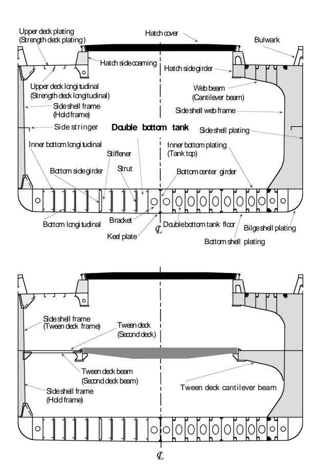
Figure 8: General Dry Cargo Ship — Typical Transverse Section
