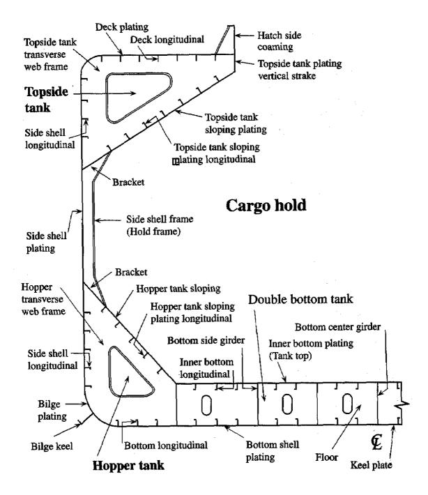
Figure 6: Single Skin Bulk Carrier — Typical Transverse Section
