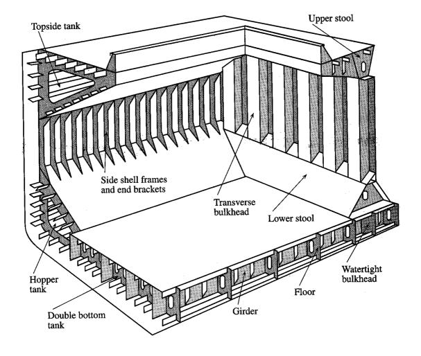
Figure 5: Single Skin Bulk Carrier — Typical Cargo Hold Structural Configuration
