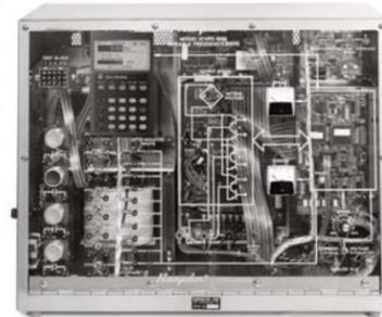
The **Model H-ACVD-PF70** Adjustable Frequency 3 $\phi$  AC Drive controls the speed of induction or synchronous motors rated to 1/2 horsepower.\* The unit is fully compatible with Hampden's Series 100 Fractional Motors and Machine program.
