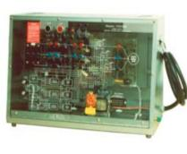
The Model H-RVS-2A 3Ø AC Reduced Voltage solid-state Starter provides students with experience in connecting. testing, and operating a commercially-available solid state reduced voltage starter for
