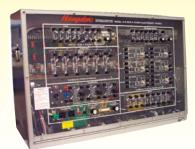
The **Model H-R-SCR-1A** provides students with the opportunity to investigate diode rectifier circuits and AC and DC controlled power circuits and unijunction transistor (UJT) triggering.
