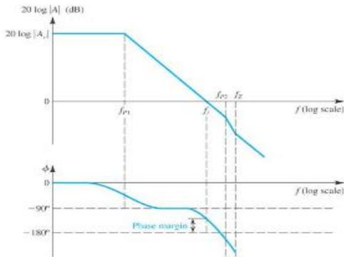
Fig.3 Bode plot of two-stage amplifier
