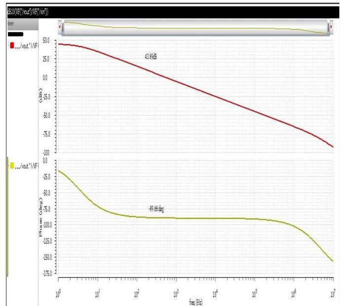
Fig.6 Phase and Gain margin of Miller Op-amp.
