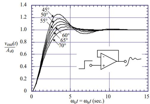
Fig. 1 Graph showing step responses of second order system
