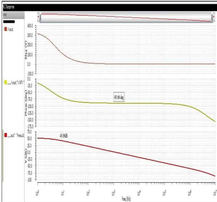
Fig.7 Phase and Gain margin of Bulk-Driven Op-amp
