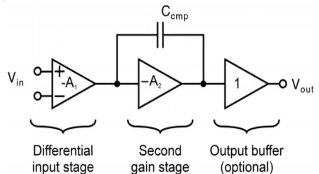
Fig.2 Block diagram of a Two-stage Op-amp
