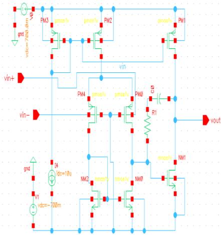
Fig.5 Bulk-Driven Op-amp
