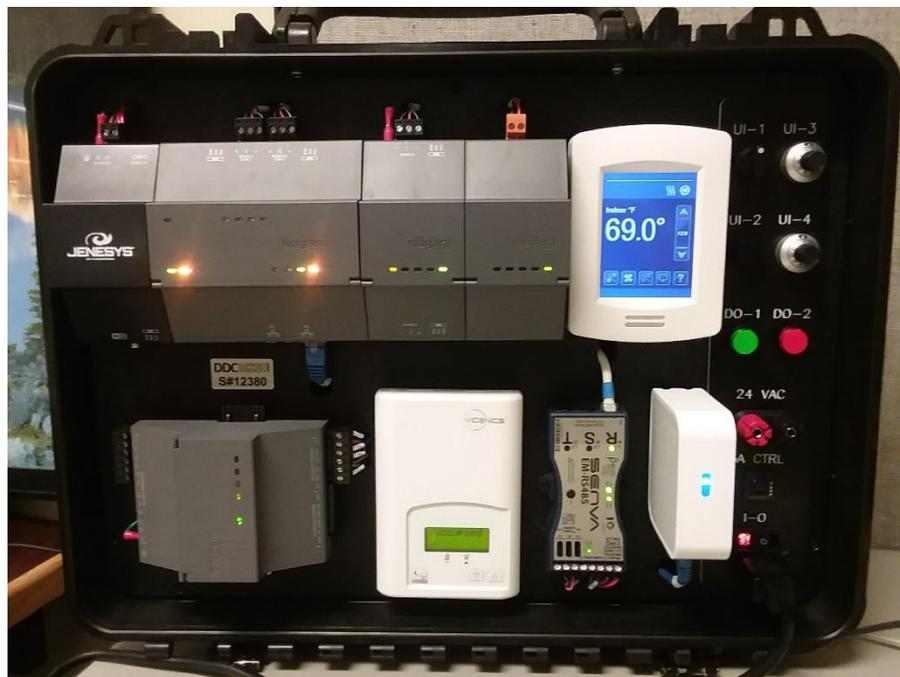
Senva EM<sup>®</sup> series meter module communicates via Modbus RTU. Three physical inputs: One push button switch, two 10k 10-turn pot and one SPST switch allow for simulation of live inputs. A TP-Link Wireless router provides wireless and hardwired Ethernet access. The PT-8000s can be operated stand alone or easily networked together for use in a learning center environment. A “Startup Demo” station
