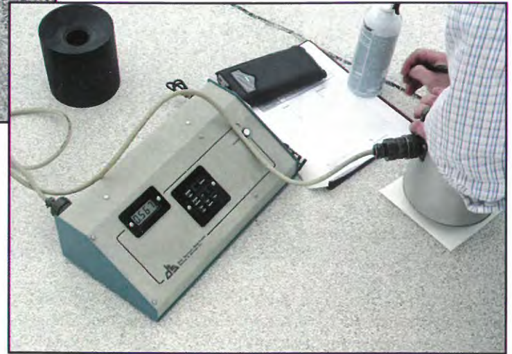
Figure 14 – Reflectivity reading of 56 on cap sheet with stained granules after exposure.
